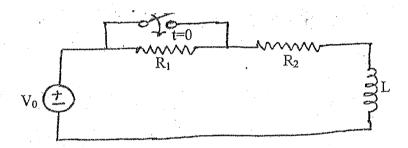
2. a) Using classical method, find the expression of current flowing through the resistor 'R' of the circuit shown in the following figure and also find the voltage across inductor 'L' for t>0.
