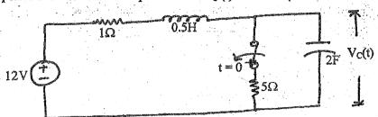
4. a) Using laplace transformation technique, find the expression for current i(t) in the network shown below for t > 0 when the switch is closed at t = 0. Assume zero initial charge across the capacitors.
