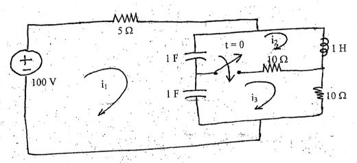
2. a) Find  $v_a(t)$  for t > 0 in the figure below using classical method.
