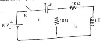
a) In the circuit of the figure below, the switch K is open and the circuit reaches a steady state. At t = 0, K is closed. Find the current in the inductor t > 0. Use classical method.
