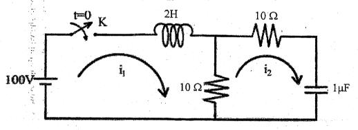
2. a) In the circuit shown in figure below, if the switch is closed at t = 0, find the expression for voltage across capacitor using classical method.
