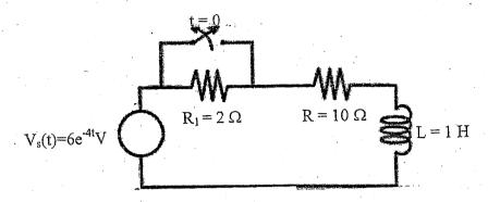
b) In the network shown in figure below, the switch is closed at t = 0, with the network previously unenergised. For the element value given on diagram, find the expression for mesh currents  $i_1(t)$  and  $i_2(t)$ , by Laplace Transformation method.
