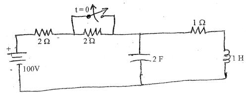
3. a) Using Laplace Transform method in the circuit shown in figure below find the voltage and current of capacitor for t > 0
