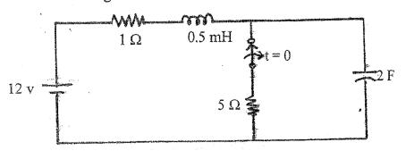
b) In the circuit shown, switch is changed from position "a" to "b" at t=0. Find the expression for current  $i_1(t)$  and  $i_2(t)$  using Laplace transformation method.
