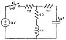
3. a) In the series R-L-C circuit shown in figure, there is no initial charge on the capacitor. If the switch S is closed at t=0, determine expression of current and voltage for all elements for t>0.
