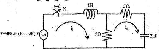
2. a) Using classical method, find the expression for the current supplied by the source in the network shown in figure. Also find the time taken by the source current to reach 25 mA.
