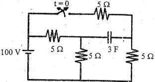
b) Switch is closed at t = 0, find the expression for circuit i(t), for any time 't', and calculate the value of current at t = 0.1 sec. Also, find the time for current reach maximum value and corresponding maximum value of current. Use Classical method.
