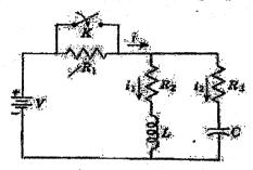
4. a) Find the forward voltage ratio transfer function  $G_{21}(s)$  and forward transfer admittance  $Y_{21}(s)$  in the following circuit.
