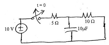
b) After being closed for a long time, if the switch in the circuit shown in figure below is opened at t = 0. Obtain the expressions for  $i_L(t)$  and  $v_c(t)$  for t > 0, using Laplace Transform Method.
