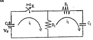
2. a) In the network shown, the switch is closed at t = 0, with the network previously unenergised. For the element values shown on the diagram, find  $i_1(t)$  and  $i_2(t)$ , by classical method for t > 0.
