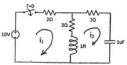
3. a) Keeping the switch at position 'a' for a long time, if the switch is moved to position 'b' at t=0 in the circuit shown in figure below, find expressions for current through and voltage across capacitor using Laplace Transform method.
