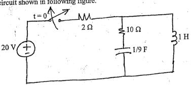
3. a) In the circuit shown in figure below, the capacitor has an initial charge of  $q_0 = 800 \,\mu\text{C}$  with polarity shown in the figure. Find current i(t) if the switch is closed at t = 0 using Laplace Transform method.
