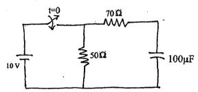
b) Find the time expression for loop currents for t > 0 in the given circuit using classical method.
