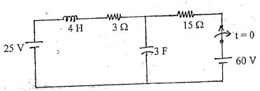
3. a) Using Laplace Transform method, find the current and voltage across inductor for t > 0 in the circuit shown in figure below.
