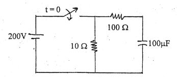
b) Keeping the switch closed for a long time, if the switch is opened at t = 0 in the circuit shown in figure below, find expression for voltage across capacitor using classical method of solution.
