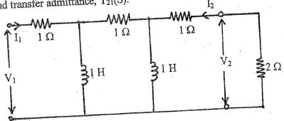
c) Express transmission (ABCD) parameters of the Two port Network in terms of Z parameters.
