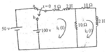
3. a) Using Laplace transform method find the current through inductor in the network shown in figure below.
