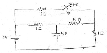
b) If the voltage source is applied at t=0 in the circuit shown in figure below, find the expression for current i(t) using transform method. Assume inductor and capacitor are initially de-energized.
