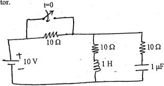
b) In the circuit shown in figure below the switch is closed at t = 0, find the expression for i<sub>1</sub>(t) and i<sub>2</sub>(t) using Laplace transform method, if the circuit is unenergised before the switch is closed.
