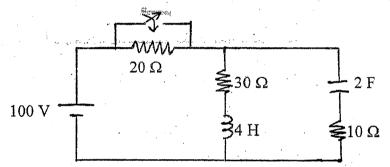
2. a) For the circuit shown in figure below, find the current through and voltage across the capacitor for t > 0. Using Classical approach.
