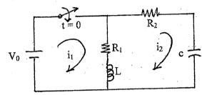
a) Using classical method, Find the current and voltage of capacitor for t > 0 in the circuit shown in figure.
