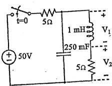
2. a) The circuit shown in figure is in the steady state with the switch S closed. The switch is opened at t=0. Determine current and voltage of all elements for t>0 using classical method.
